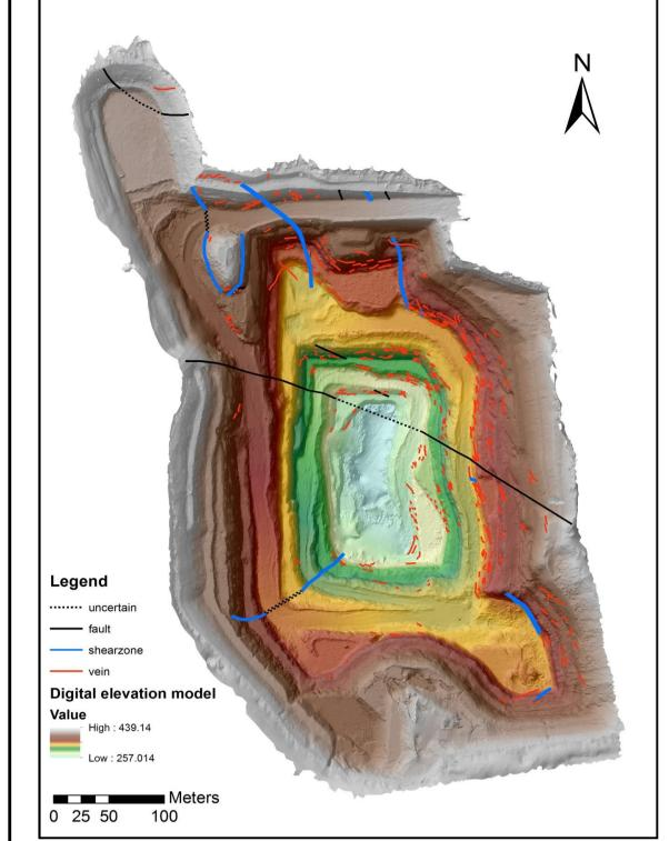
— fault dolerite photographic Fig 13. Digital maps produced in ArcGIS,
