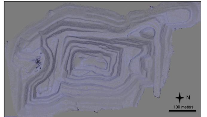
Fig 7. Geometric construction of a three dimensional wireframe model having total of 158353 faces.
