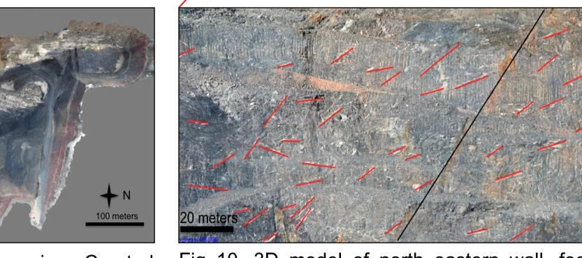
Fig 10. 3D model of north eastern wall, focal length: 50mm. Veins (red) and fault (black) marked
