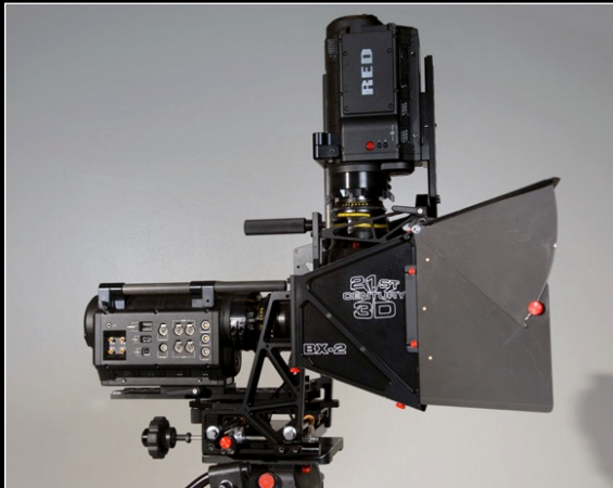
21st Century 3D camera using a beamsplitter (2010)
