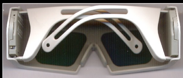
Typical emitter and frame sequential shutter glasses
