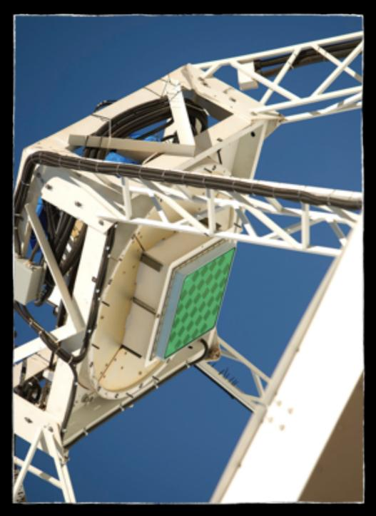
Chequer board sensor array on each dish
