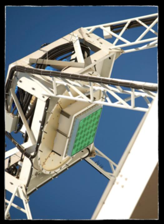
Chequer board sensor array on each dish
