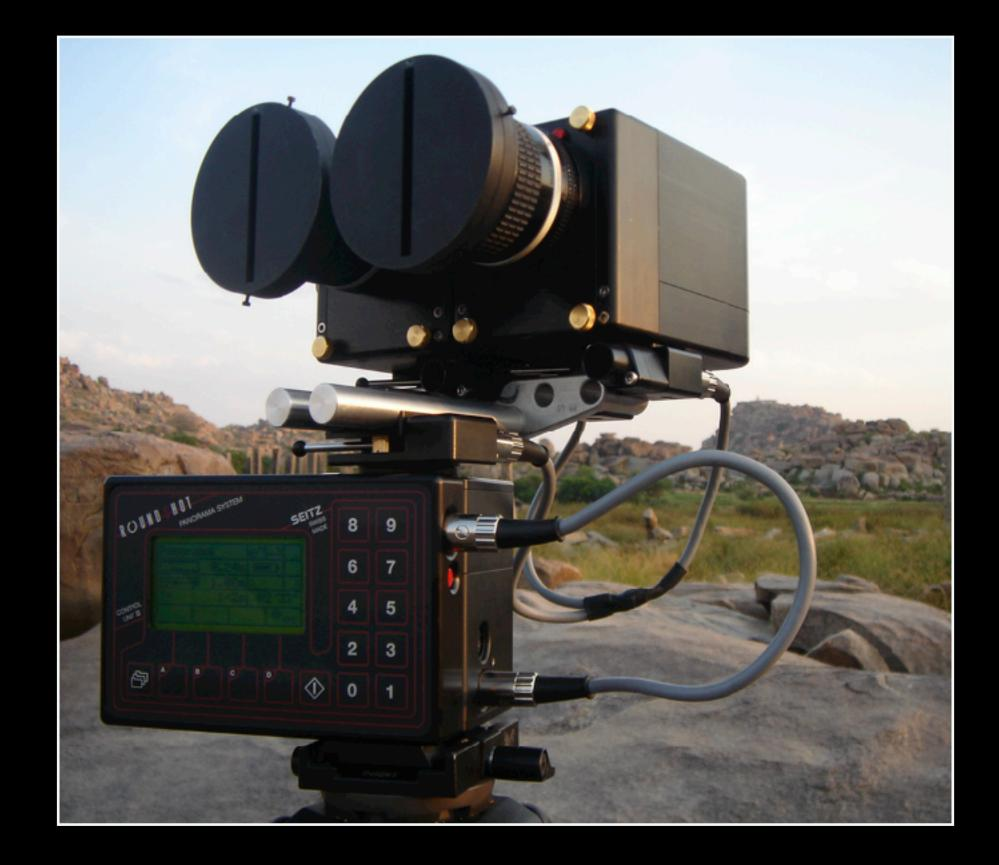
Exposure controlled by rate of rotation, fast in high light, slow in low light. Fixed slit width and only one film stock, only other exposure control is lens aperture.
