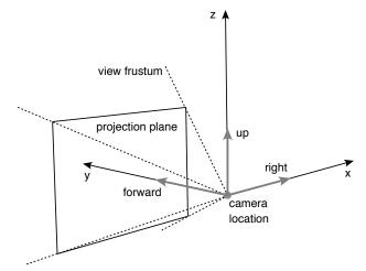
To create a particular perspective view one rotates this initial camera direction and orientation about any axis, or combination of axes. A roll in the chosen coordinate system is a rotation about the y axis (forward), panning is a rotation about the z axis (up) and tilting is a rotation about the x axis (right). To create the 6 faces of the cube map the initial camera view direction is rotated as shown, the horizontal and vertical field of view set to 90 degrees.
