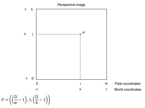
3. Rotate this vector P about the axes corresponding to roll, tilt and yaw to orientate the perspective camera as desired, call this vector P'
