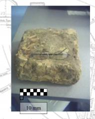
Fig. 3 photograph of an unfired brick taken in Crossley's lab
