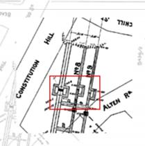
Fig. 6 enlargement of Altern Rd entrance to tunnel complex with three 'baffles' encompassed inside red box
